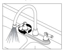
Figure 10 - Let the hot water run until it is cool.
