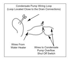
Figure 15 - Wiring Loop for connection to Condensate Pump.
