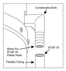
Figure 4 - Condensate drain connection
