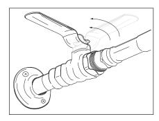
Figure 11 - Cold water supply in OFF position.
