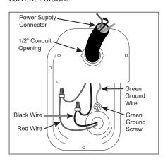
Figure 23 - Connecting the electrical wires (bottom cover to electrical junction box removed for clarity).
