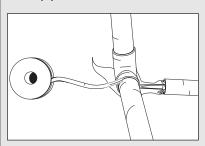
Solder a short length of pipe (about 12"/30 cm or so) to a threaded adapter using only 95/5 tin-antimony or equivalent solder. Attach the threaded adaptors to the water heater's connections (using thread sealant tape or pipe joint compound). Connect the home's water pipes by soldering, keeping the connections at the water heater cool with wet rags. **DO NOT** over apply joint compound.
