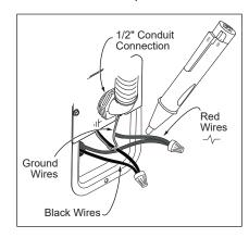
Figure 46 - Non-Contact Circuit Tester.
