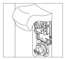
Figure 50 - Element Access Panel/ECO Compartment.
