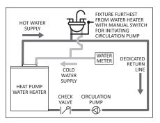
Figure 20 - Recirculation Loop Diagram with Manual Switch.
