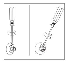
Figure 12 - Draining the old water heater.
