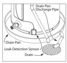
Figure 7 - A suitable drain pan piped to an adequate drain can help protect flooring from leaks and drips.
