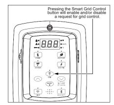
Figure 32 - Smart Grid Control Button
