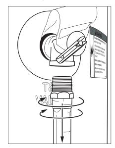
Figure 13 - Removing the T&P Relief Valve discharge pipe.
