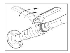
Figure 22 - Fully open the cold water supply valve (full-flow ball valve pictured above).
