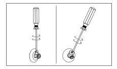
Figure 39 - Open Drain Valve.
