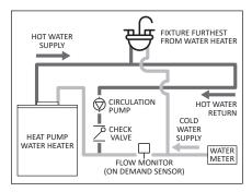
Figure 21 - Recirculation Loop Diagram with Sensor Control.
