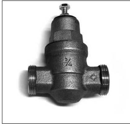
Figure 15 - A Pressure Reducing Valve is required if your home's water pressure is above 80 psi (552 kPa).
