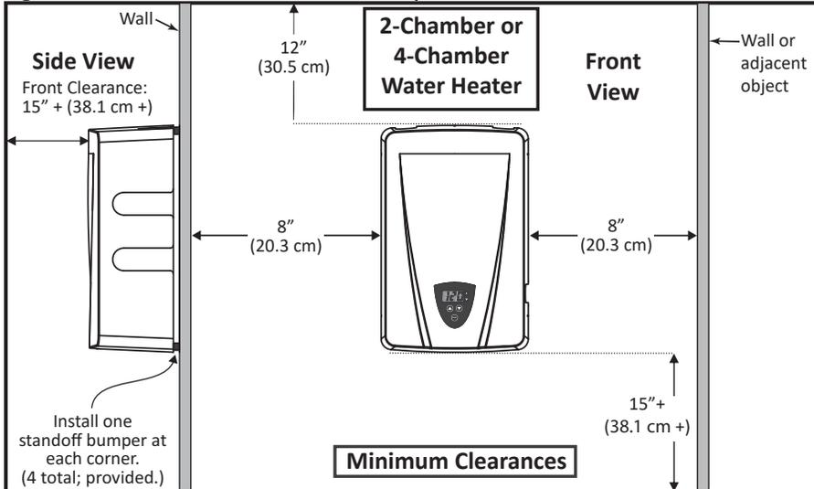
**Side Clearance:** Allow an 8 inch (20.3 cm) minimum horizontal space for the heater. This horizontal clearance will allow for the removal of protective cover screws and provide access to electrical wires that will enter the heater from the side.
