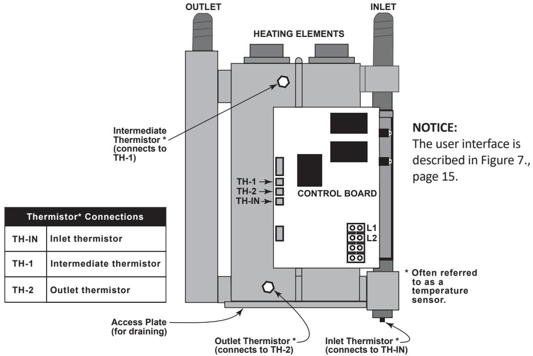
Component Identification: Four-Chamber Models (R4L, C4L, R4M, C4M)
