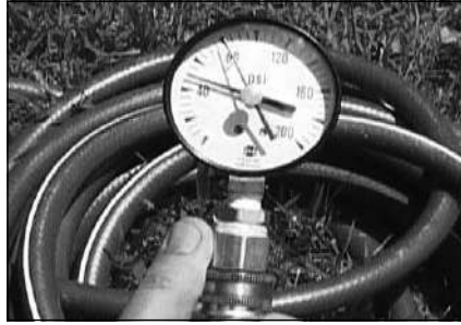
Figure 6 - Use a Water Pressure Gauge to make sure your home's water pressure is not too high.
