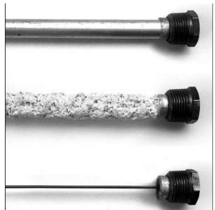
Figure 33 - Anode Rods from new (top) to partially depleted (middle) to fully depleted staged (bottom)
