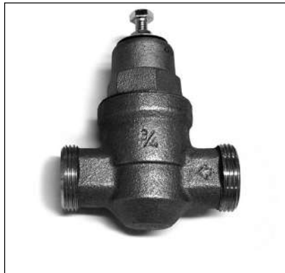
Figure 18 - A Pressure Reducing Valve is required if your home's water pressure is above 80 psi/550kPa.
