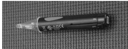
Figure 27 - Use a non-contact circuit tester to check for electrical power.
