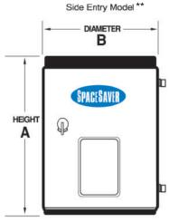
\*\*Note: 6, 12 and 19 USG models have side connections on left of unit.
