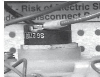
Figure 11. Installed heating element
